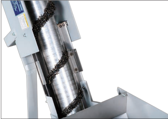
SCC/SC chip discharge
